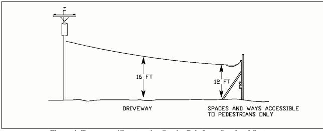
Figure 4: Temporary/Construction Service Pole from Overhead System
