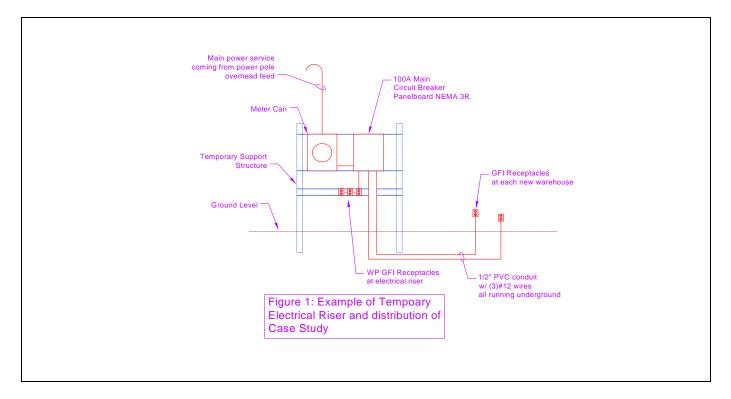
Figure 1: Example of Temporary Electrical Riser and Distribution for Case Study
