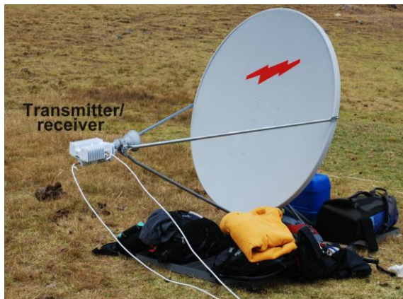
Figure 4: Satellite antenna with transmitter and receiver
