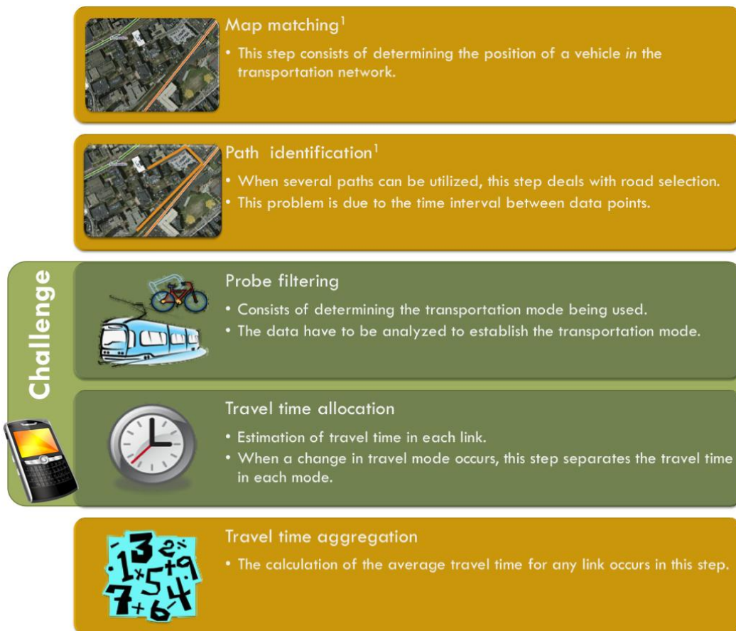
Figure 1: Determining traffic conditions from positioning data 1
