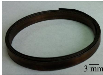
Figure 4. Steel 1020 strip produced by LSEM for \gamma = 2 , p_{OA}/k = 2.5 and V = 60 m/min (before heat treatment). Thickness = 0.15 mm, width = 3 mm.
