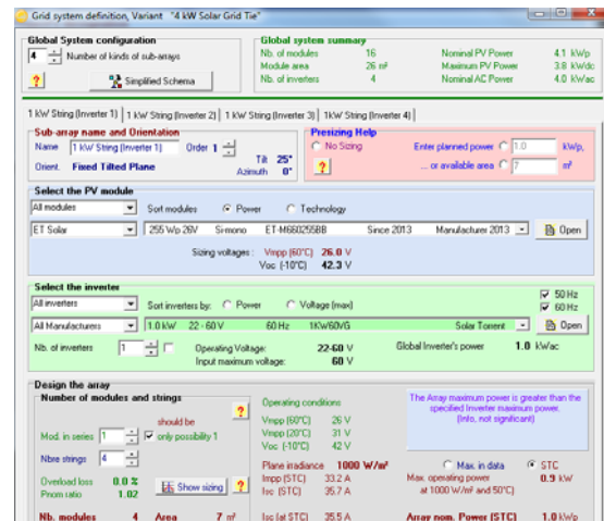
Figure 9: 4 kW Grid Tie Equipment Configuration
