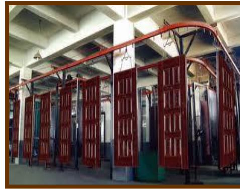
Figure 2: Track and spray system of an industrial automated powder coating machine
