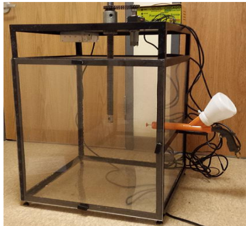
Figure 4: Plexiglas chamber of designed powder coating machine
