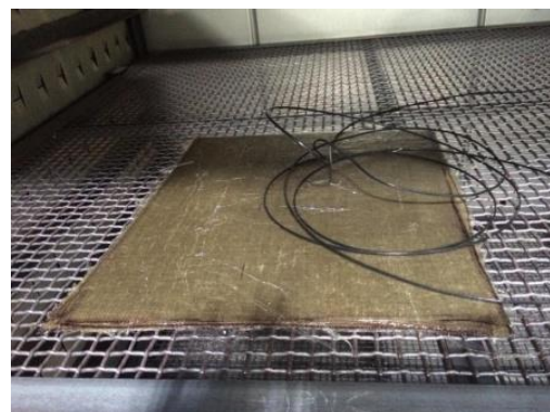
Figure 10 - Post cure in oven at 120°F for two hours
