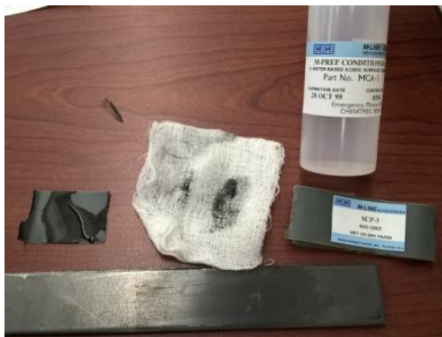
Figure 12 - Surface after conditioner and 400-grit sandpaper
