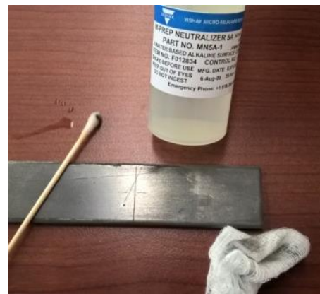
Figure 13 - Neutralizer applied with cotton swab
