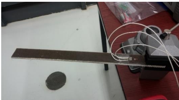
Figure 18 - Clamped flax-epoxy specimen
