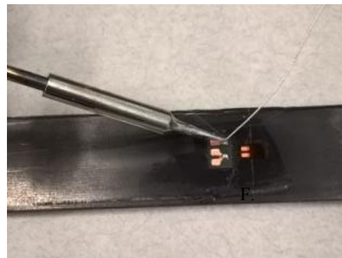
Figure 15 - Soldering strain gauge to terminal
