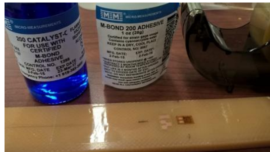
Figure 14 - Bonding catalyst and adhesive with strain gauge and terminal prepped on glass-epoxy coupon
