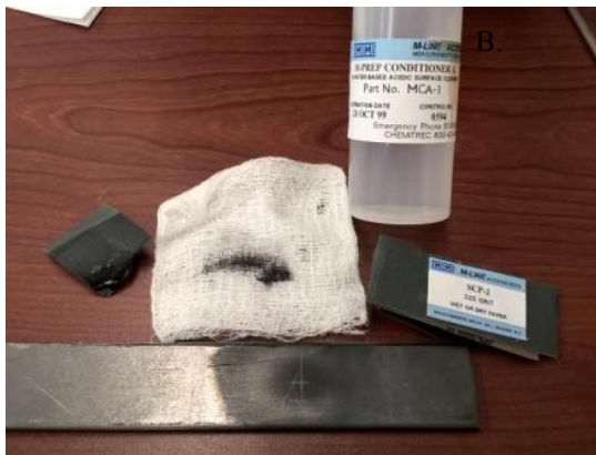
Figure 11 - Surface after conditioner and 320-grit sandpaper
