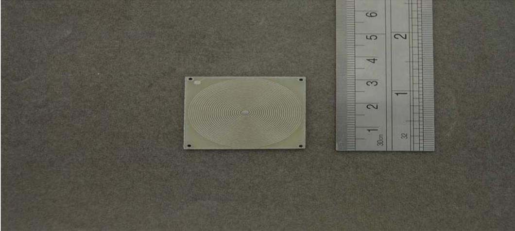
**Pic01:Corless PCB Transformer No. 1**
