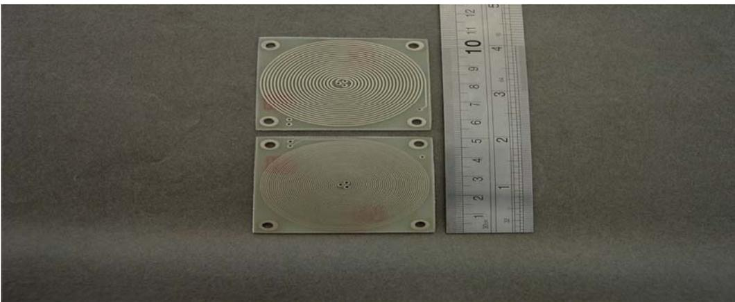
**Pic03:Corless PCB Transformer No.3**
