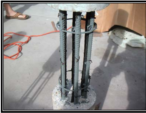
Figure 13: Specimen Spliced with FRP
