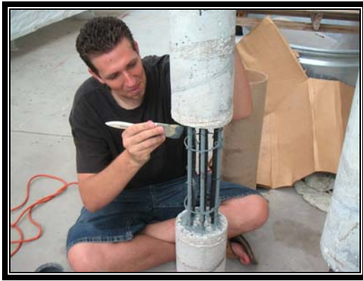
Figure 6: Reinforcement coating with rebar primer
