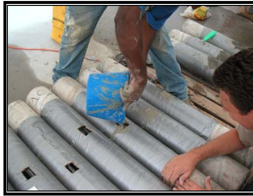
Figure 9: Mix Pouring for Repair 2
