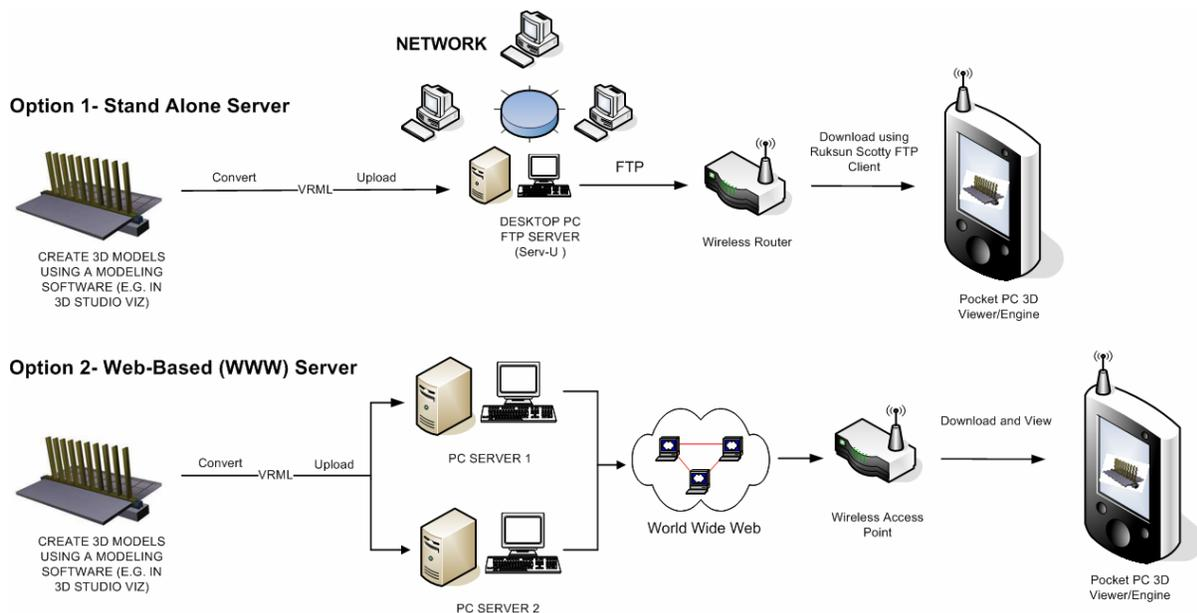
Figure 5: Framework for Wireless 3D Visualization in the Classroom Using the Pocket PC (Perdomo et. al. (2005))
