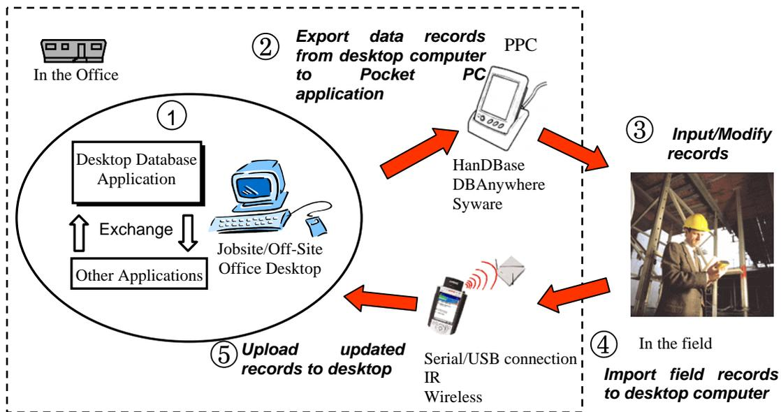
Figure 2: Automation of field data collection using PocketPC
