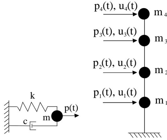
Figure 3. a) SDOF System. b) MDOF System.
