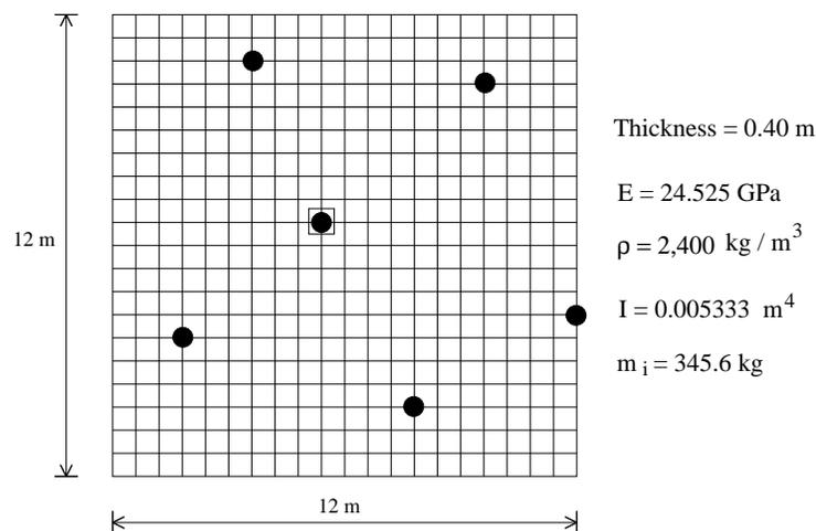
Figure 5. Plate dimensions and data for example problem.
