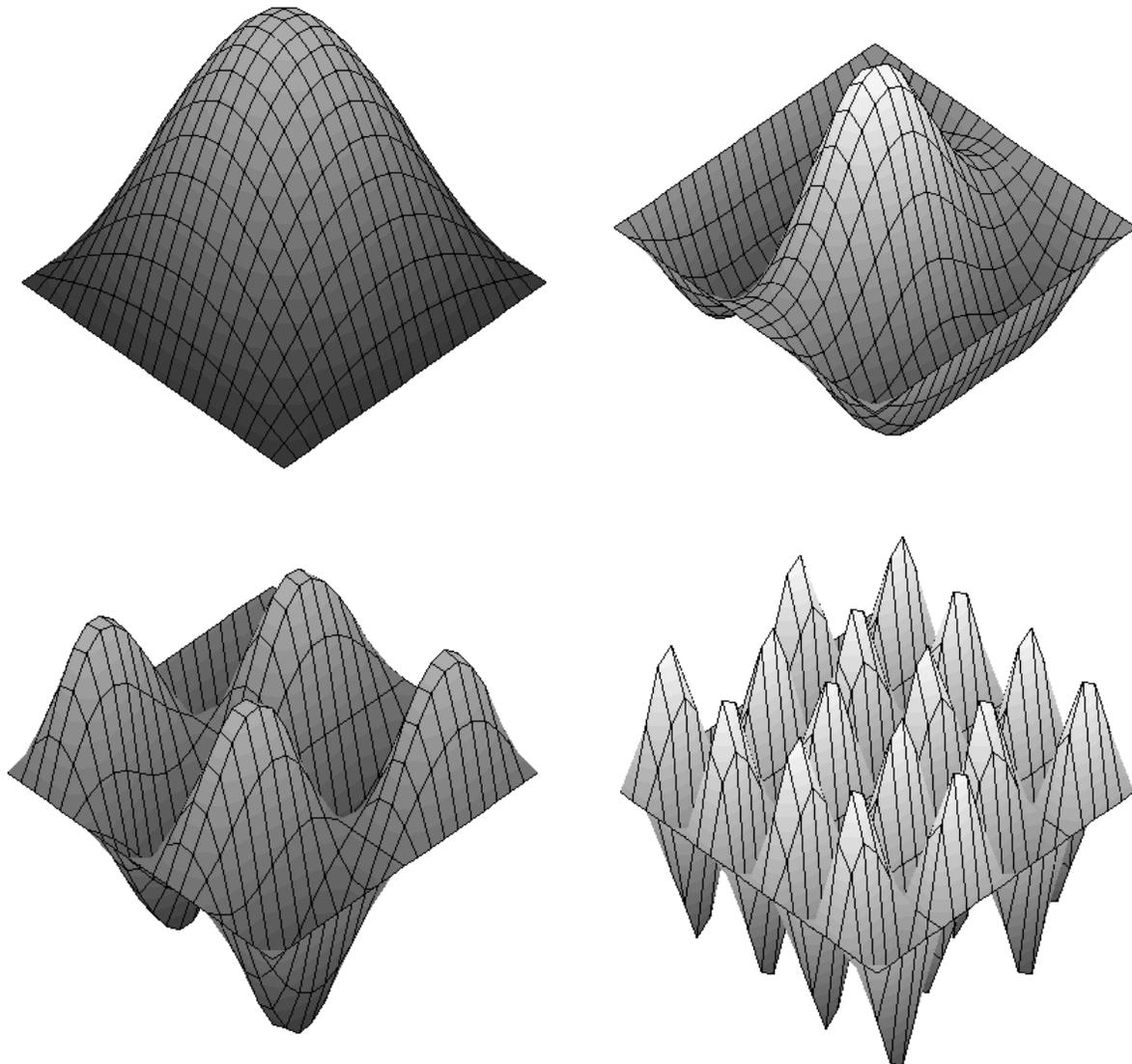
**Figure 7. Clockwise From Top to Bottom: Modes of Vibration 1, 4, 12, and 55.**
