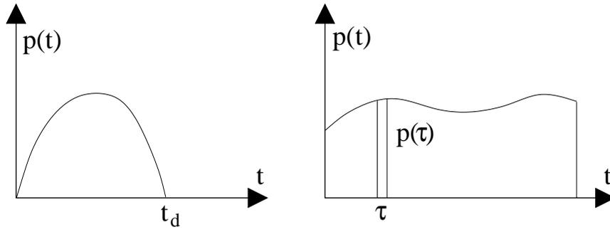
**Figure 4. a) Impulse load. b) General dynamic load.**
