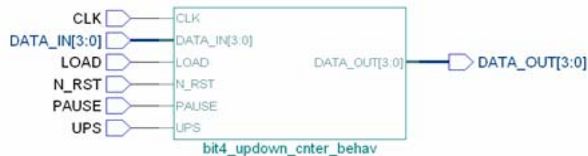
Figure 2: 4-bit Up-Down counter Architecture Description
