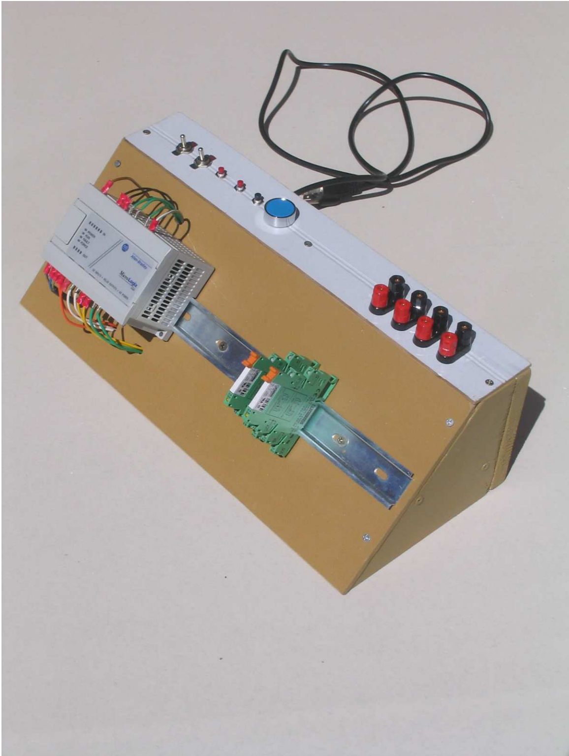
Figure 2: PLC station hosting Allen Bradley MicroLogix 1000 unit and relay units-Side View
