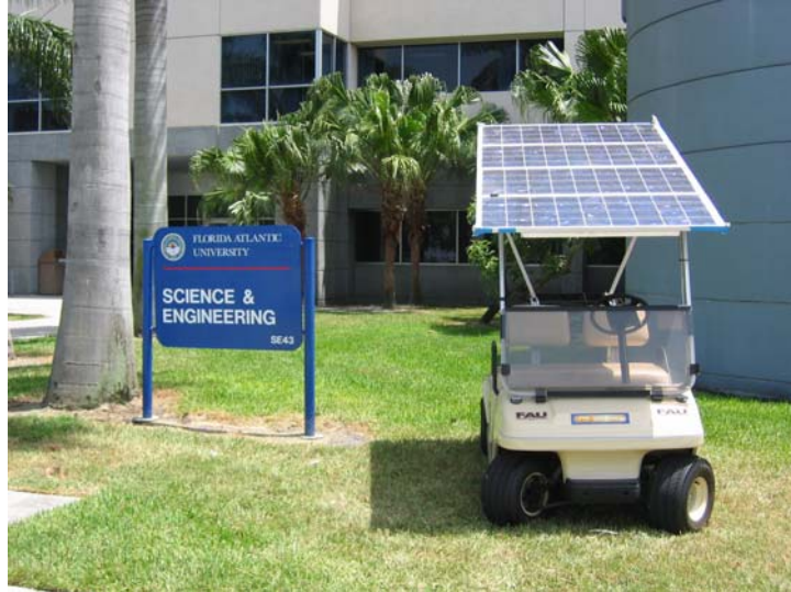
Fig1. The solar golf cart collecting energy to charge the batteries
