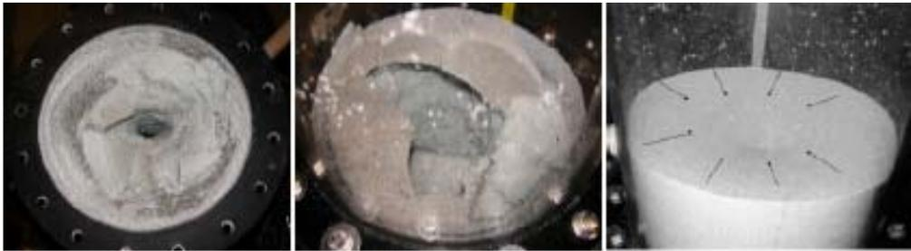
**Figure 8: Throttling vertical tube failed to prevent funnel flow in the absence of double pyramid insert.**
