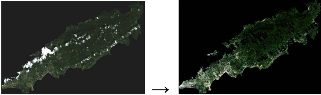
**Figure 1: Cloud and Cloud Shadow masking of the Landsat ETM+ 2001 scene.**
