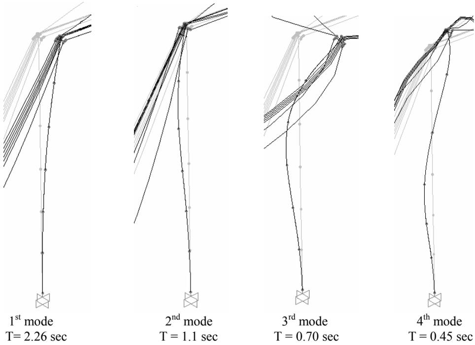
**Figure 9: First four flexural modes of tower T8**
