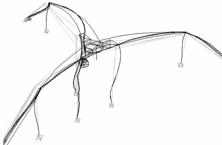
**Figure 12: Deformed geometry (100x magnification), 6.2 sec into the Morgan Hill earthquake**
