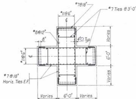
**Figure 4: Cruciform shape of tower cross-section (courtesy of NAIC)**
