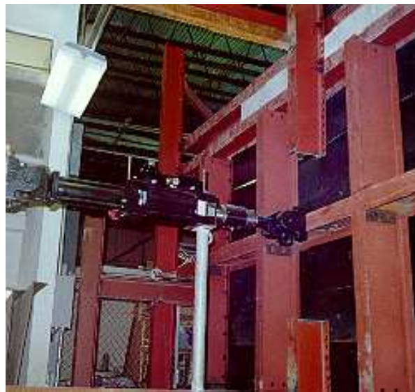
Figure 6. Final Assembly: Load Transfer System
