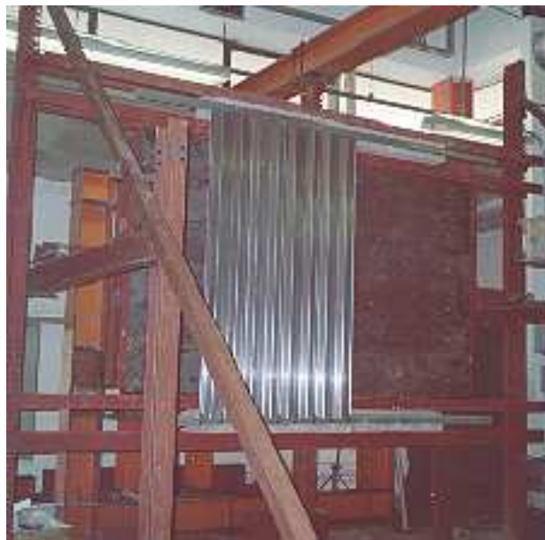
Figure 4. Final Assembly: Rigid frame with the shutter
