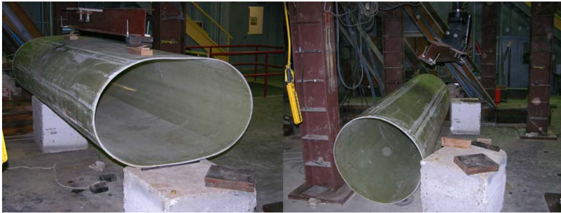
Figure 11: Left-13in Deflection on 37.25in Pipe. Right-Pipe Pull Out and Returns to Original Shape.
