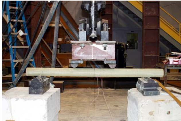
Figure 3: Load – Deformation Test Setup for 3in Pipes
