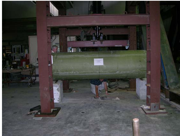
Figure 9: Load - Deformation Test Setup for 37.25in Pipes
