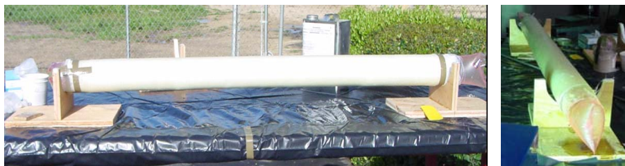
Figure 2: Left-Beam 1 Begins Curing in Sunlight. Right-Curing with UV Lamp.
