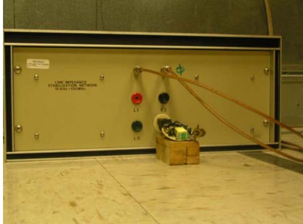
Photograph 2: The CP SPS Conducted Measurement Setup
