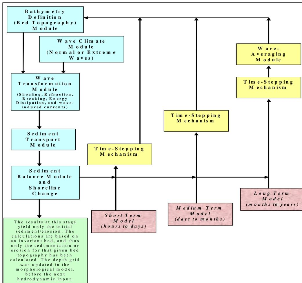
**Figure 1 Interaction Diagram showing the modules of the proposed numerical model**
