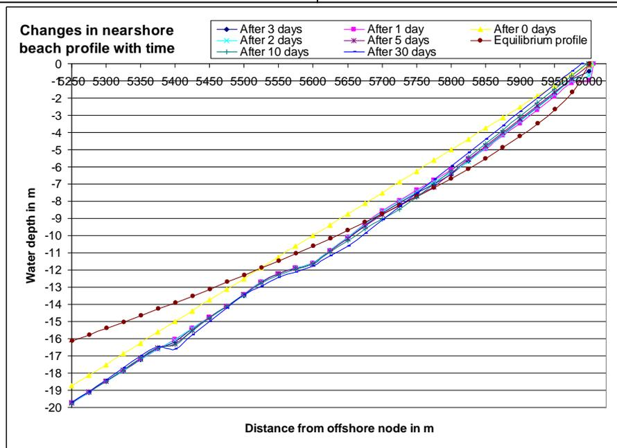
(c) Graph showing changes in nearshore beach profile for the various simulation lengths during the hurricane periods
