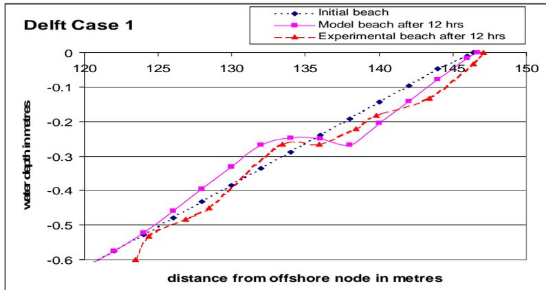
**Figure 5 Comparison of the profile change of the model beach with the experimental results after 12 hours**
