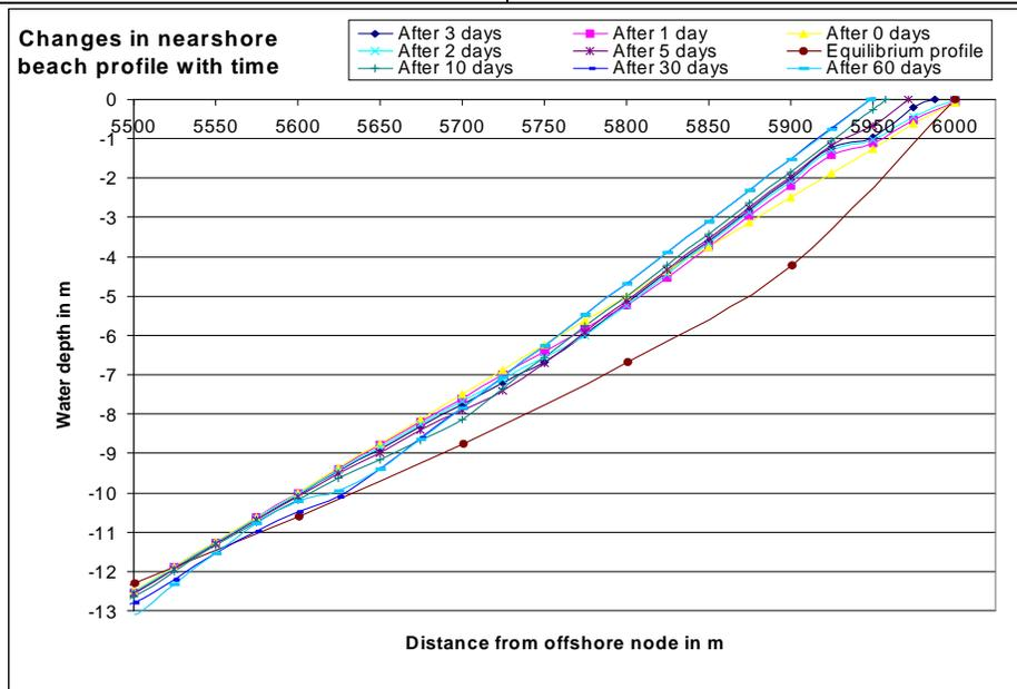
(c) Graph showing changes in nearshore beach profile for the various simulation lengths during the non-hurricane periods
