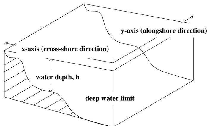
**Figure 2** Co-ordinate axis system used in the numerical morphological model
