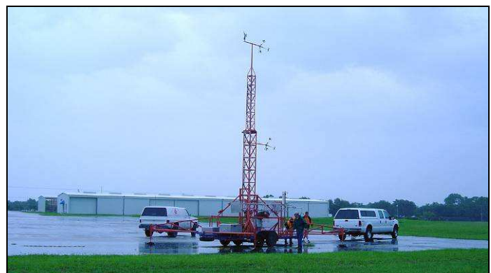
Figure 1: FCMP mobile tower in tow, and tower deployed during Charley (2004) in Plant City, FL
