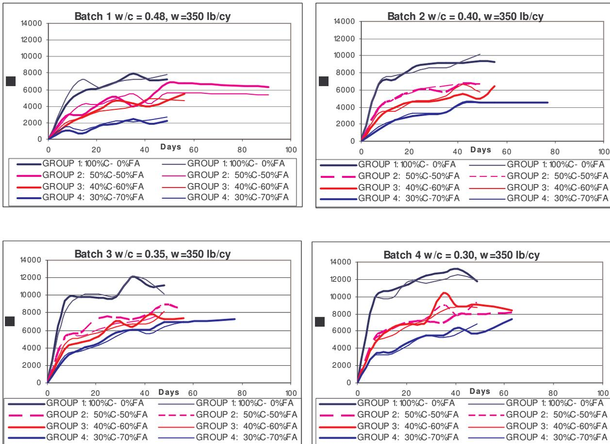
Figure 1: Compression strength versus time for concretes with different w/c ratio and a water content of 350 lb/cy.
