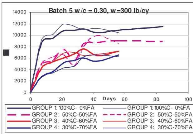
**Figure 2: Compression strength versus time for concretes with different w/c ratio and a water content of 300 lb/cy.**
