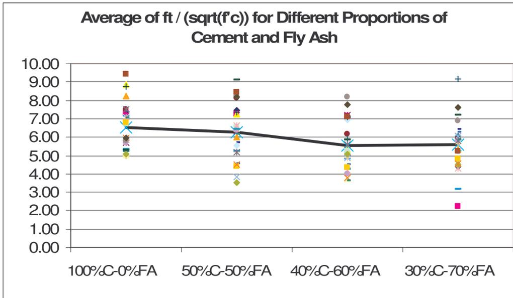
Figure 4: Variation of the ratio of tension and square root of compression strength with the fly ash content
