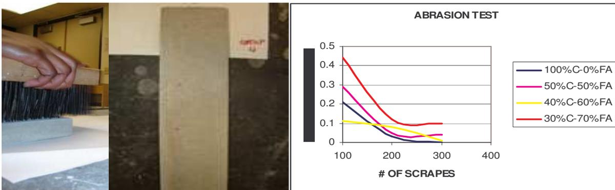
Figure 5: Scrapping test performed to a concrete plate to simulate the abrasion effect on concrete with different proportion of fly ash.
