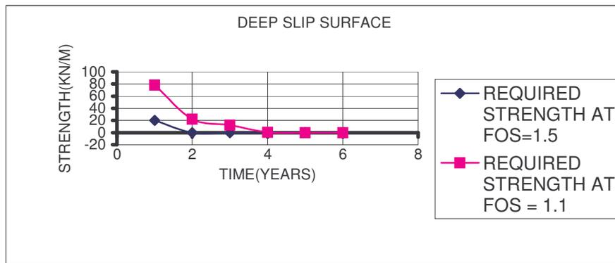
**Figure 3. Reinforcement strength required maintain a specified Factor of Safety**
