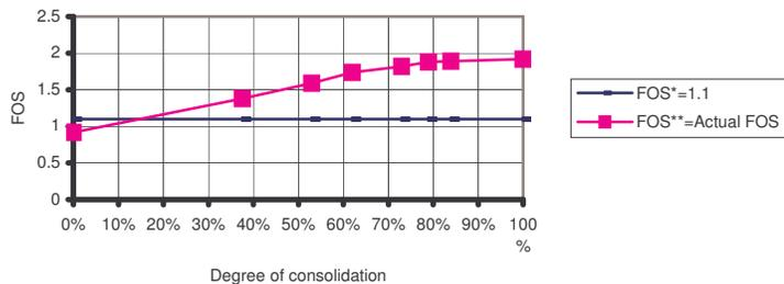
**Figure 2 Effect of consolidation on Factor of Safety**
