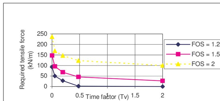
**Figure 5 Estimation of required reinforcement strength with varying Time Factor (Tv) at critical slip surface ( $D_{cc}/D = 0.67$ , 1 m beyond the toe)**
