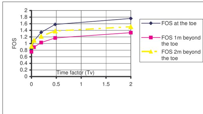
**Figure 4 Variation of FOS with Time Factor (Tv) at various depth ratio ( $D_{cc}/D$ )**
