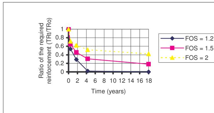
**Figure 6 Proportion of reinforcement strength with time (at critical slip surface  $D_{cc}/D = 0.67$ . 1m beyond the toe)**
