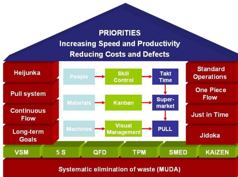
**Figure 1: Main Principles and Tools applied by Galgano Group for implementing a Lean Production System**
