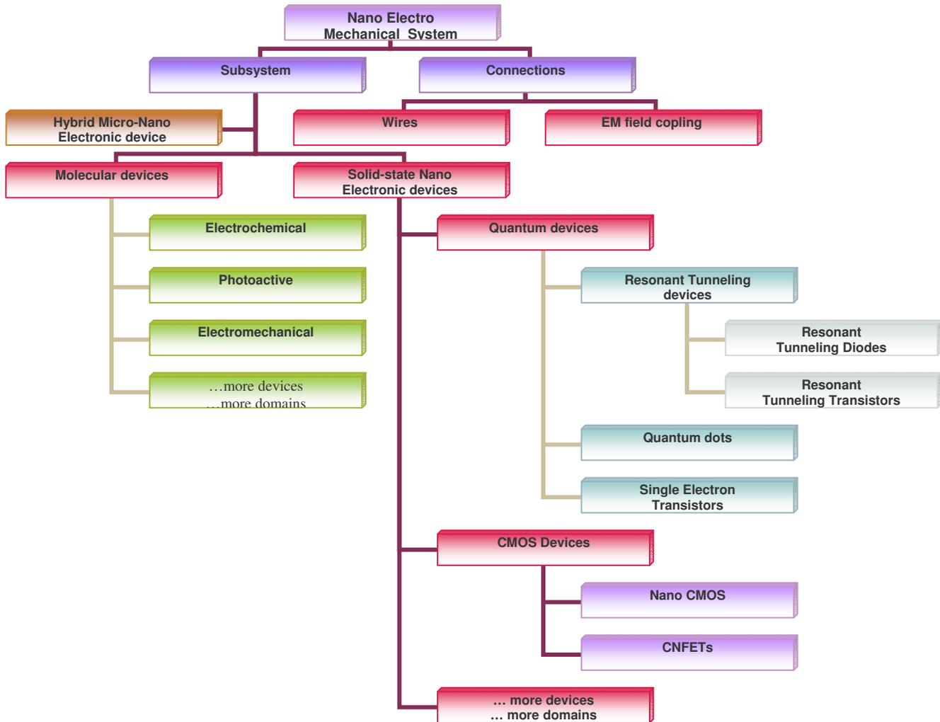
**Figure 1.: Hierarchical organization of nanodevices for NEMS**
