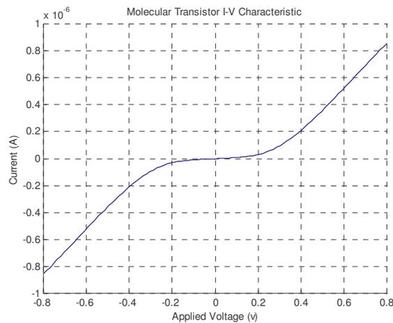
**Figure 4. Detailed view of Molecular Transistor I-V characteristic.**
