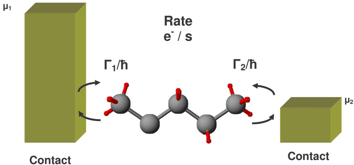
Figure 2: Schematic view of a molecular transistor model.
