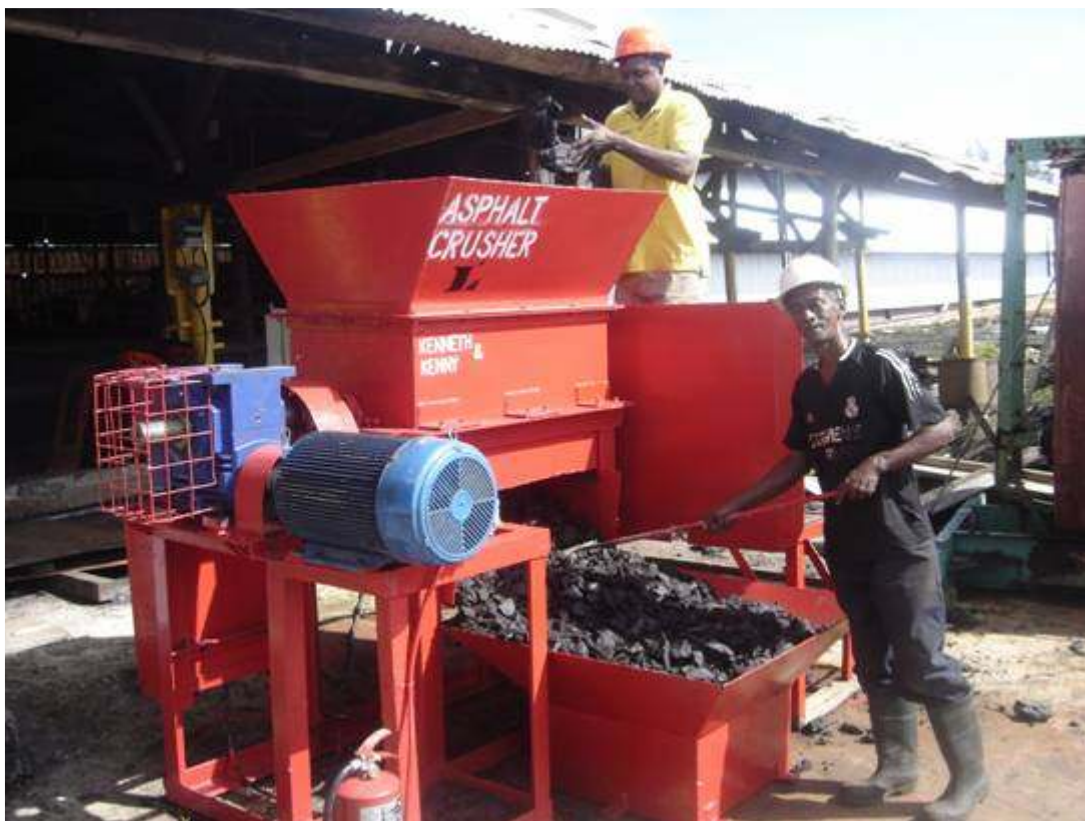
Figure 5 Fully functional crude asphalt crusher
