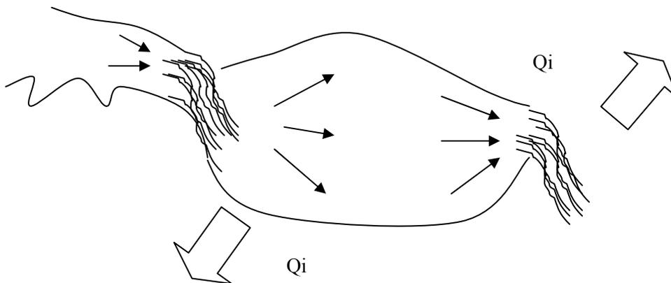
**Figure 4: Kinetic and potential energy interchanges producing losses**
