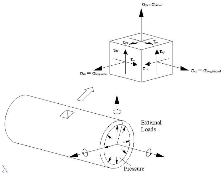
**Fig. 4: Free body diagram showing the combined loading and stresses acting on a body**
