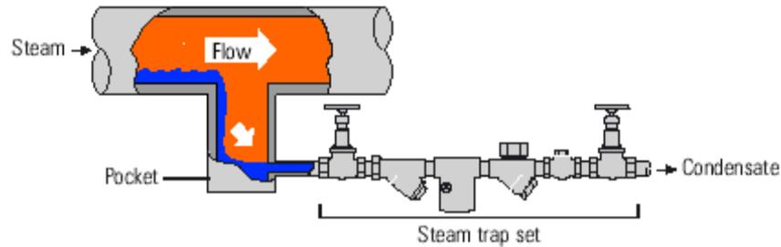
**Fig. 10: Properly sized trap pocket**
