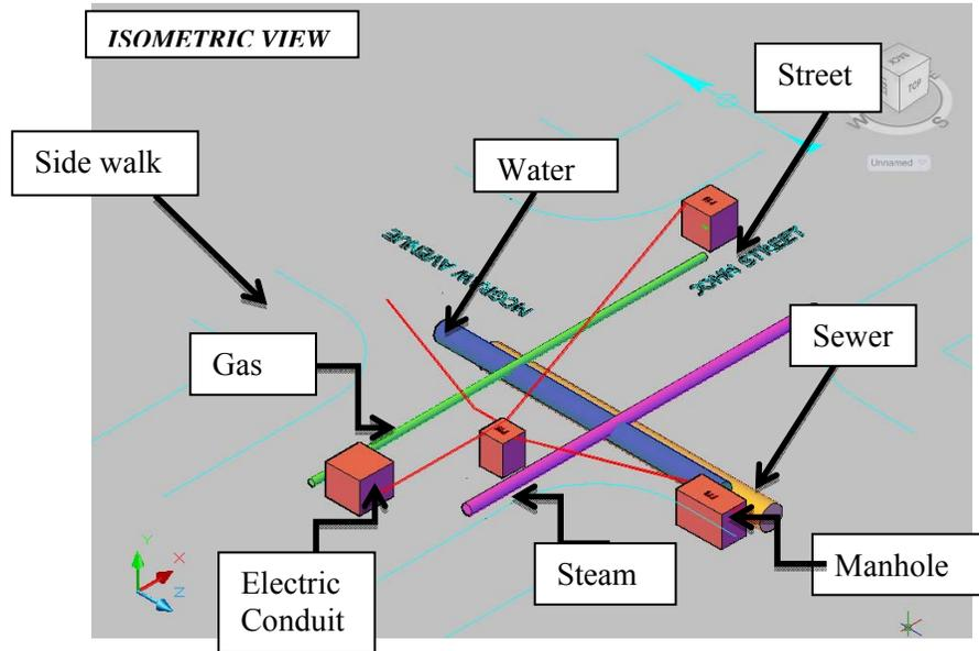
**Fig. 3: AUTOCAD 3D model Projection of the existing case of the steam pipe with interference**
