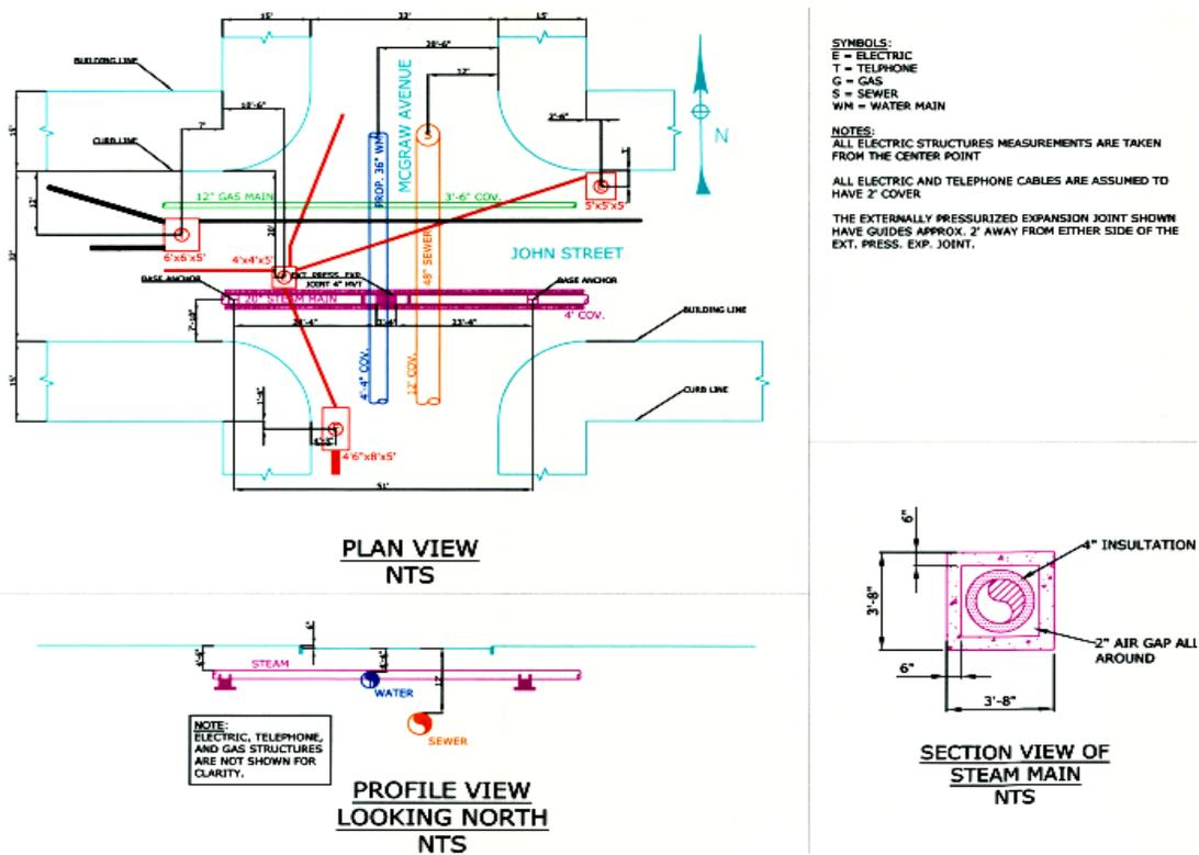
**Fig. 2: Technical drawing showing the steam main in direct interference with the water main**
