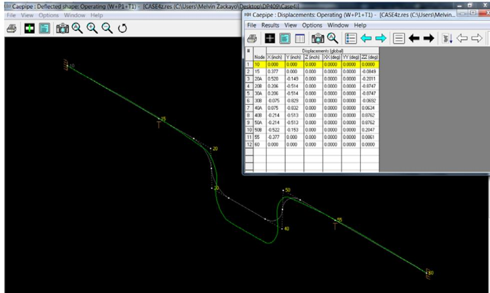
**Fig. 9: CAEPIPE results: Operating displacement.**
