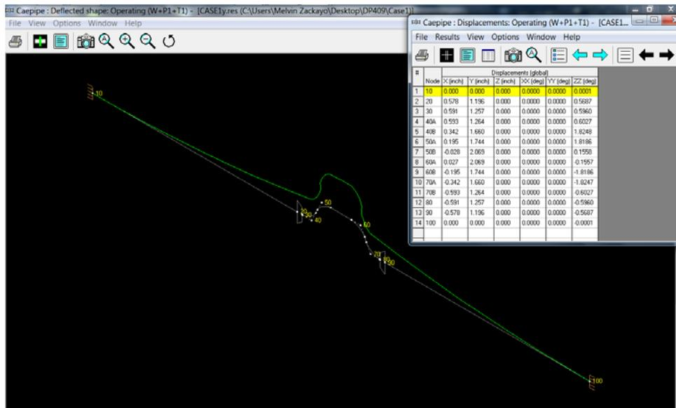
**Fig. 7: CAEPIPE results: Operating displacement.**
