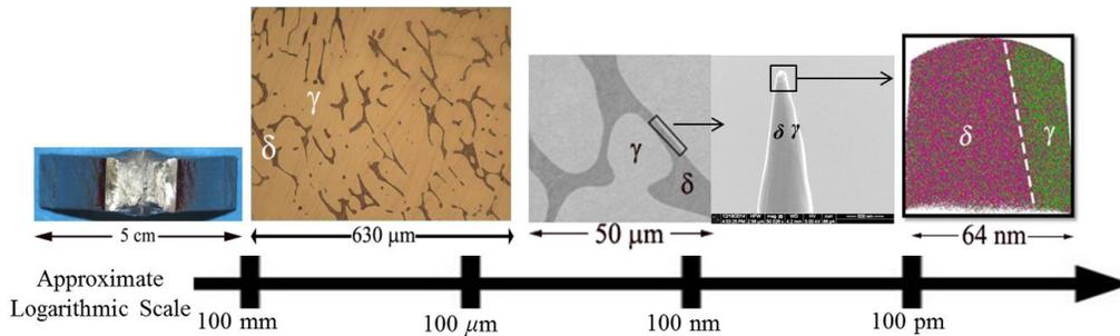
Fig. 1. Experimental procedures across multiple length scales leading to atomic level analysis: APT reconstruction of unaged CF-3, depicting 30% of the Cr ions (magenta), and 100% of Ni (green) and C (black) ions for clarity.
