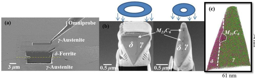
Fig. 2. (a) The *in situ* site-specific lift-out of an APT sample at the  $\delta$ -ferrite/ $\gamma$ -austenite heterophase interface (dashed yellow line) using a SEM/FIB instrument. (b) Series of images illustrating annular milling of a specimen into needle morphology with subsequently decreasing tip diameter necessary for APT analysis. (c) The APT reconstruction of unaged CF-8, depicting 30% of the Cr ions (magenta), and 100% of Ni (green) and C (black) ions for clarity.
