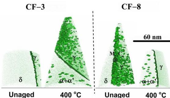
Fig. 3. The APT reconstructions of CF-3 and CF-8 steels' ferrite phase that are unaged ( $\delta$ ) and thermally aged ( $\alpha+\alpha'$ ) to 4300 hours at 400 °C illustrate G-phase precipitates in the aged samples.
