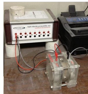
Figure 2. Specimen mounted between the hollow cells
