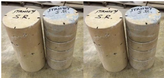
Figure 4. Sound and cut specimens for Surface Resistivity Testing
