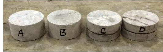
Figure 1. Sound and cut specimens for RCP testing
