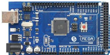
Figura 4. Arduino MEGA 2560. [8]
